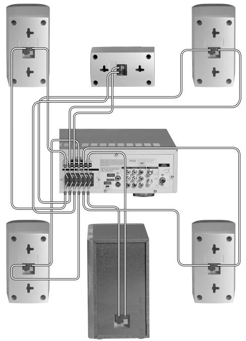
**CAUTION**: Short circuits may damage the system. Make sure the exposed tip of each speaker wire does not touch another speaker wire or terminal.
